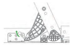
In the case of a power cut or unexpected breakdown, the mechanical emergency levelling function makes it possible to lower both the dorsal and foot sections manually.
